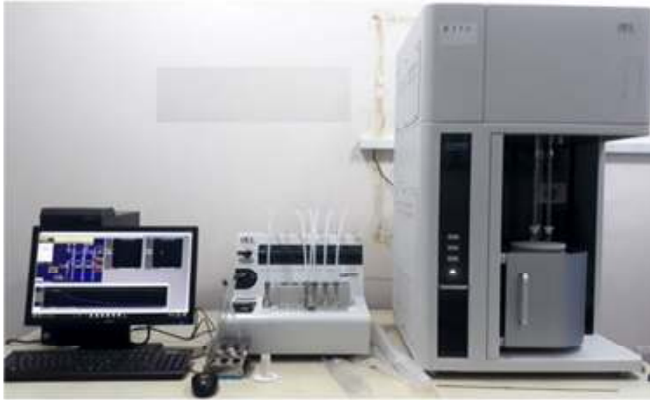
Picture of BET surface area and pore size analyzer installed in VISTAS
